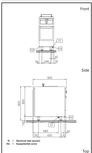
Electric Supply voltage: 400 V/3N ph/50/60 Hz Total Watts: 10 kW **Key Information:** Number of wells: Usable well dimensions (width): 240 mm Usable well dimensions 225 mm (height): Usable well dimensions 380 mm (depth): Well capacity: 12 lt MIN; 14 lt MAX Thermostat Range: 100 °C MIN; 180 °C MAX External dimensions, Width: 400 mm External dimensions, Depth: 900 mm External dimensions, Height: 800 mm Net weight: 75 kg On Base;One-Side
